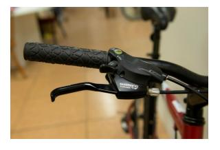
The handle bar tube is structurally undamaged. Handlebar grips are present and in good condition. The gear and brake cables are securely attached with no fraying.
