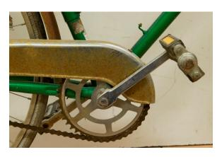
Significant rust can be found on the cranks, pedals, chainrings, mudguard and chain guard. The time and effort required to fix this severely undermines the value of this bike as a donation.
