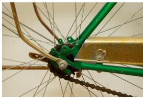
This bicycle has significant rust on most of its components. The drivetrain is dry and rusty, as are the stand, carrier and chain guard. This takes significant resources to remedy.
