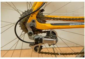
The derailleur, despite being old, is free of significant rust and is securely attached. In this case, the chain has some rust and is showing signs of significant wear.
