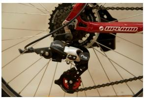
The derailleur and gear cluster are in good condition with no rust. The gear cable is securely attached with no fraying. No missing, broken or rusted spokes.
