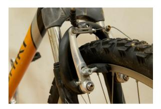
The brake components are intact, although out of alignment. There is some surface rust. The pads are significantly worn, but still have some useful life. Similarly, the tyre tread is worn with some useful life.
